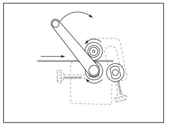
Figure 18. Feeding the workpiece.
